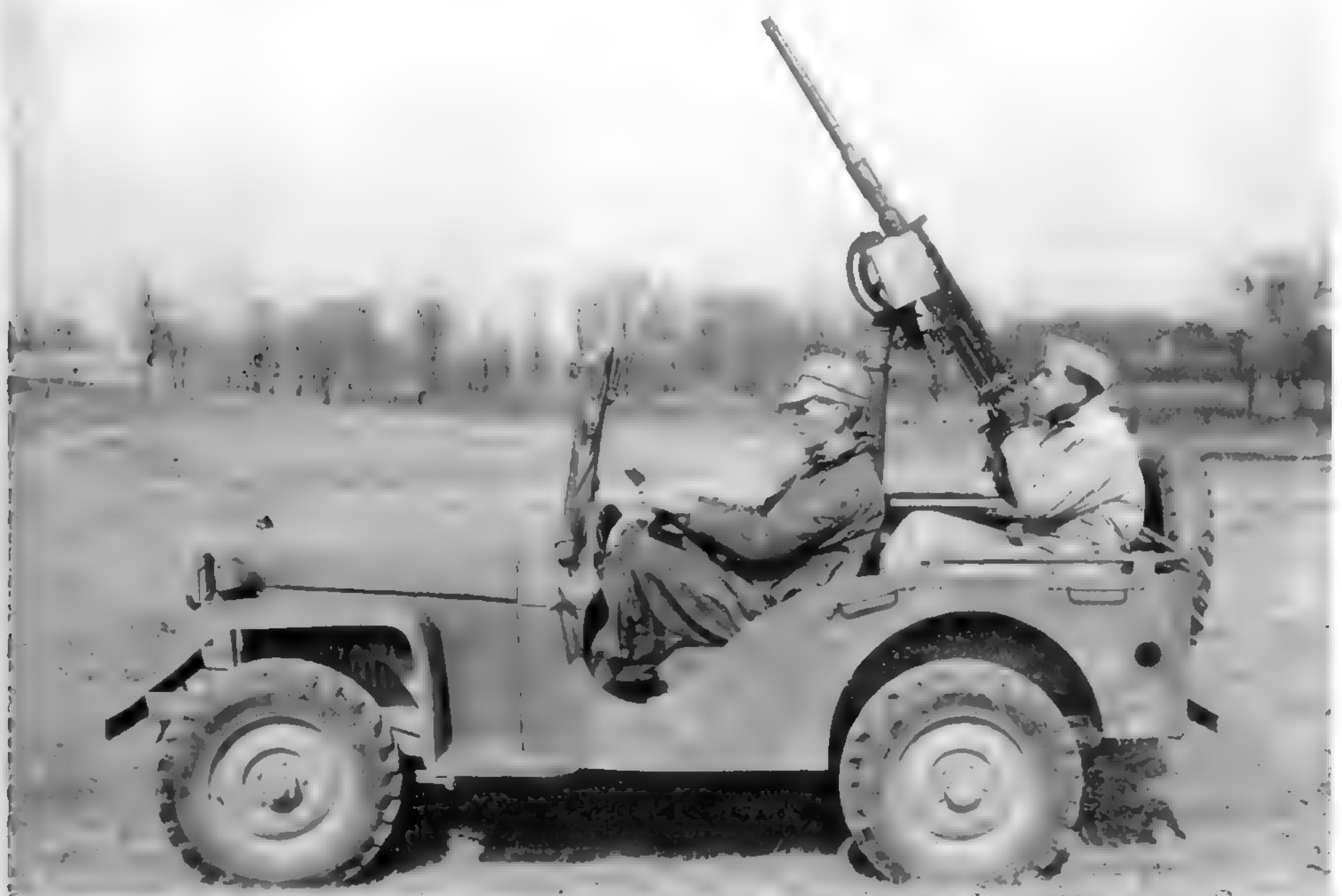
The 69 vehicles that were built on the pilot contract were known as the Bantam Model 60. This one was photographed at Aberdeen Proving Grounds in March 1941 outfitted with a machine gun. The scalloped doorway of the prototype has been replaced with a simpler opening, just as the elaborate fenders have been replaced with these simple flat versions. (Photo courtesy of the Patton Museum)
